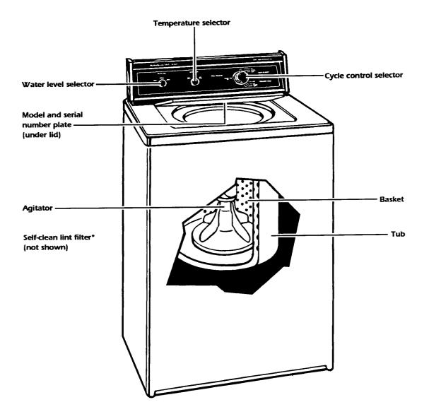
\*As load is washed and rinsed, lint particles automatically collect on the SELF-CLEAN LINT FILTER located between the basket and tub. Collected lint is carried away with the wash and rinse water as the washer drains. If the washer drains into a tub, remove any lint collected in the drain or strainer.
